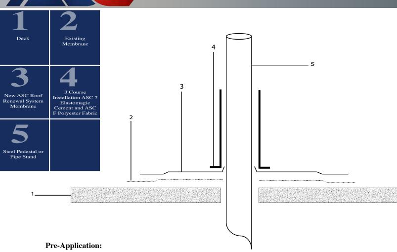
Surfaces must be structurally sound, cleaned, dried, and free of moisture on and beneath the surface. Remove all dust, dirt, oil, loose granules and any other foreign contaminants. Remove any other loose, flaking or existing waterproof coatings, which may affect the adhesion. Rusted metal should be cleaned with a wire brush.
